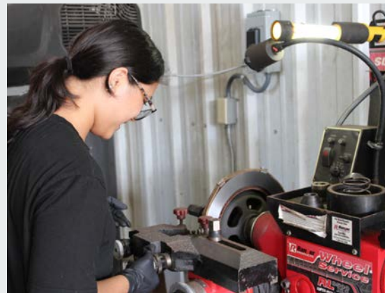
Our Automotive Technology students learned the proper procedures and safety measures to resurface disc brakes.
